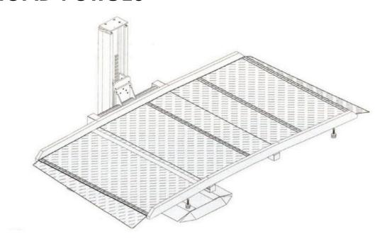
Loading on the ground x 2000kg = 10,45 KN/MQ Loading on the ground x 2000kg = 13,06 KN/MQ
